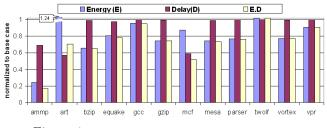
Figure 4: PA-CDRAM energy-delay break down.
