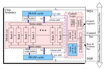
Figure 3: Functional block diagram of a PA-CDRAM.
