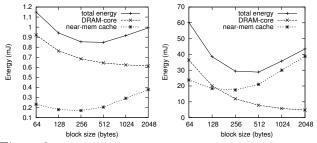
Figure 2: The effect of varying the cache block size on the memory energy consumption for *bzip* (left) and *mcf* (right).
