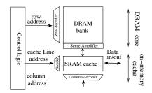
Figure 1: Functional block diagram of a CDRAM
